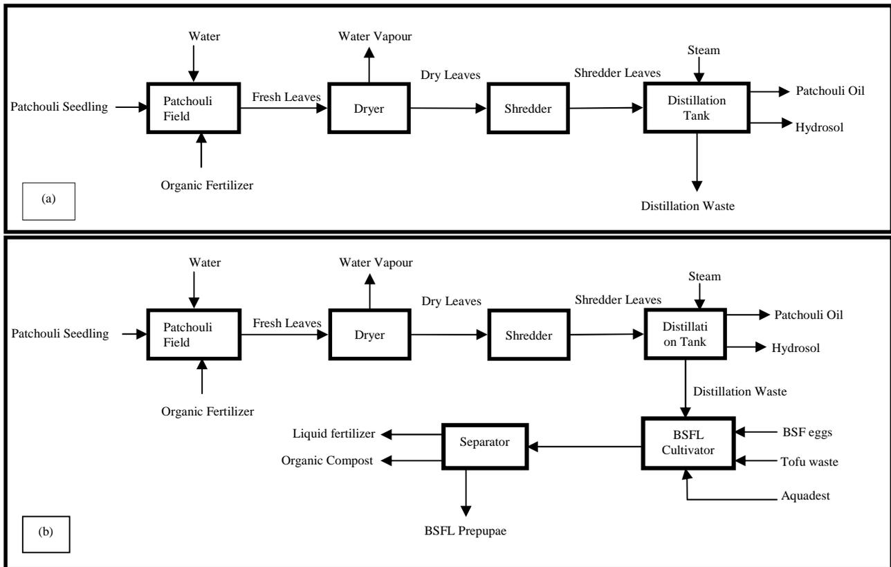
Fig. 1. Production scheme by using (a) Conventional process and (b) Biorefinery concept
