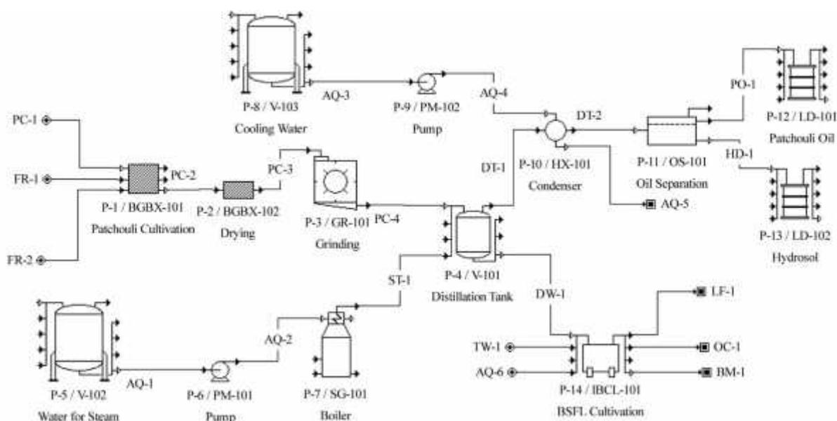
Fig. 3. Process flow diagram of the production system
